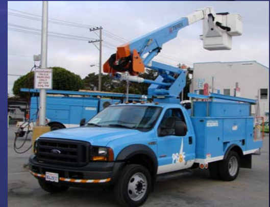
Eaton/Ford/EPRI F-550 Super Duty Trouble Truck
